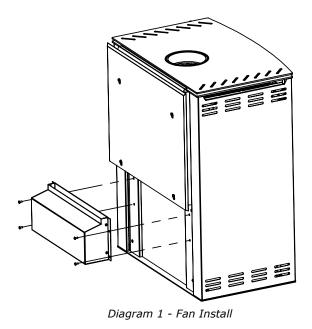
A 2 speed fan is supplied and needs to be fitted to the rear of the unit with screws supplied.
