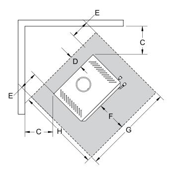
The flue pipe shall extend not less than 4.6m above the top of the floor protector.
